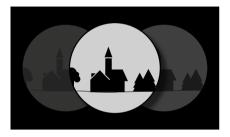
Adjust the interocular distance by moving the hinged joint to match your personal requirements. When the interocular distance is set correctly, the right and left fields of view merge into a circular image.
