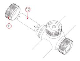
special label in the battery compartment designed for it, that is, the positive pole faces inward and the negative pole faces outward.
