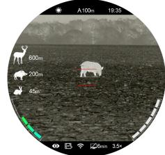
display area. Rotate the rotary encoder (7) clockwise to enlarge or anticlockwise to reduce the width of the measurement lines, so that the target is completely between the measurement lines. While adjusting the width of the measurement lines, the rangefinder values on the right change accordingly.
