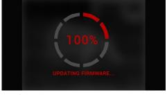
10. Please delete the Firmware file off of the microSD card after the process is complete. Or the system will try to update the Firmware every time you turn the monocular on.
