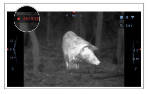
While recording the Counter widget appears. In order to Start recording video. While on the Homescreen, Press the RIGHT button to activate video recording. Press the RIGHT button once more to Stop recording video.
