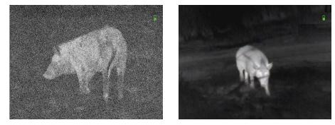
NUC'ing helps to improve the image quality when the image is degraded by various environmental factors. There are multiple NUC tables that span the full operating temperature range, and the monocular automatically selects the optimum table based on its temperature.
