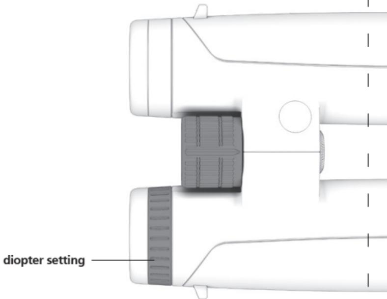
Cover or close your LEFT eye. Using the diopter adjustment ring, focus your RIGHT eye on your selected object until the picture is sharp.
