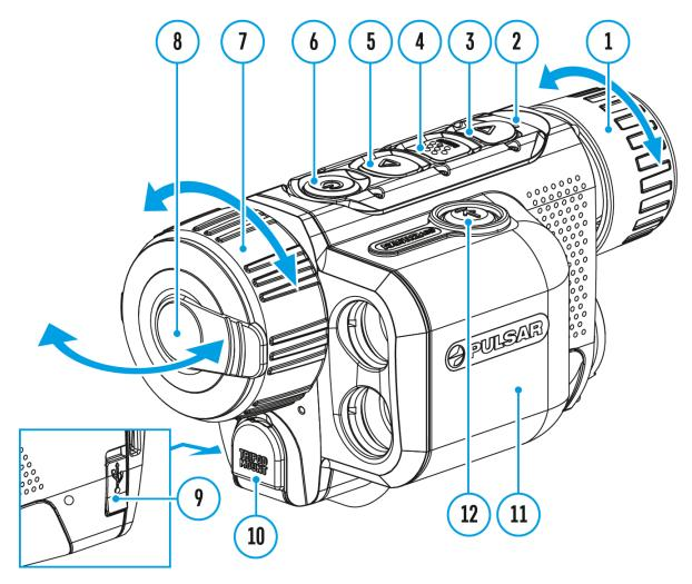
The **Axion 2 LRF** thermal imager is equipped with an integrated laser rangefinder.
