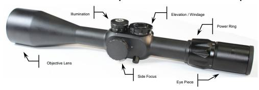
**FFP Brief Introduction:** The scopes fit the reticle in the first focal plane. The reticle increases its size when change the magnification from low to high. The advantage with telemetric reticles (like rangefinder & Mil-dot etc) is that the target image and distance between dots remains constant even when changing magnification.
