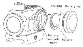
Fig 2 Battery Installation
