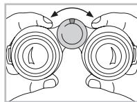
By turning the focusing wheel you can sharply focus the object you are observing.
